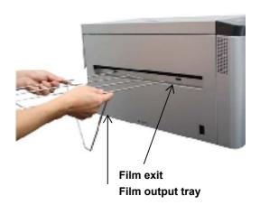
2. While slightly widening the film output tray, insert the other claw into the other mounting hole.
