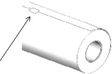
Install and fit the flange (anti-gear side) to 6. the end of the shaft on the opposite side of the film.
